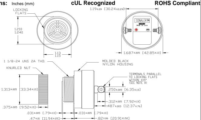
NOTE A: TERMINALS-,032 BRASS TIN PLATED, TAPPED FOR #6-32 SCREW. TWO #6-32 NICKEL PLATED BRASS SCREWS INCLUDED, WILL ACCEPT 1/4"
