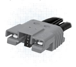
SBE® and SBO® connectors build on the capability of the two pole SB® connectors by offering up to 8 auxiliary power / signal contacts along with an IEC 60950 touch safe housing. The center of the main connector features a connector holder for either: two PP15-45, two PPMX, or APP's innovative 1x4 auxiliary connector.
