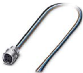
Sensor/actuator flush-type socket, 4-pos., M8, front/screw mounting with M8 thread, with 0.5 m PVC litz wire, 4 x 0.25 mm 2
