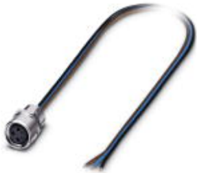
Sensor/actuator flush-type socket, 3-pos., M8, front/screw mounting, with M8 thread, with 0.5 m TPE litz wire, 3 x 0.25 mm 2
