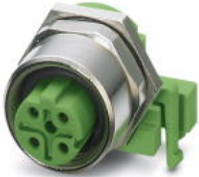
Bus system flush-type socket, ETHERNET, 4-pos., M12, shielded, D-coded, rear/screw mounting, with angled solder connection
