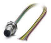
Sensor/actuator flush-type plug, 8-pos., M12-SPEEDCON, rear/screw mounting with Pg9 thread, with 0.5 m TPE litz wire,  $8 \times 0.25 \text{ mm}^2$
