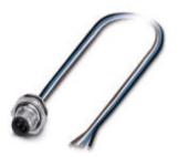
Sensor/actuator flush-type plug, 4-pos., M12 SPEEDCON, rear/screw mounting with M16 thread, with 0.5 m TPE litz wire,  $4 \times 0.34$  mm<sup>2</sup>
