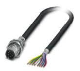
Flush-type plug, shielded, 8-pos., M12, A-coded, rear/screw mounting with M16 thread, with 1 m cable, 8 x 0.25 mm<sup>2</sup>
