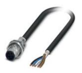
Flush-type plug, shielded, 5-pos., M12, A-coded, rear/screw mounting with M16 thread, with 2 m cable,  $5 \times 0.34$  mm<sup>2</sup>
