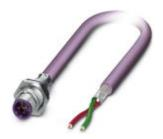
Bus system flush-type plug, PROFIBUS, 2-pos., M12, shielded, B-coded, rear/screw mounting with M16 thread, with 2 m bus cable, 2 x 0.25 mm<sup>2</sup>
