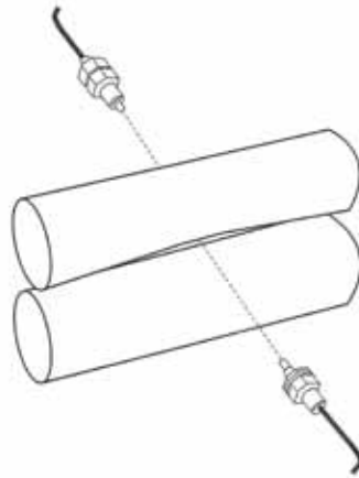
Detecting the roundness of rollers
