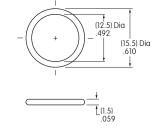
1 included with each switch Material: Brass with tin-cobalt alloy plating 1 included with each switch
