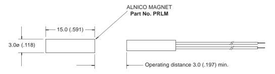
Drawings not to scale All dimensions in mm (inches) nominal Different magnets will give varying operating distances.
