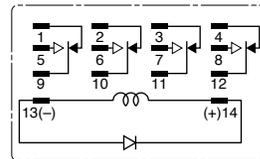
Contains a diode to absorb the back emf generated when the coil is de-energized. The release time is slightly longer.
