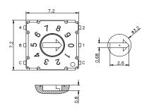
1 Slotted Spindle (Height = 3 mm)
