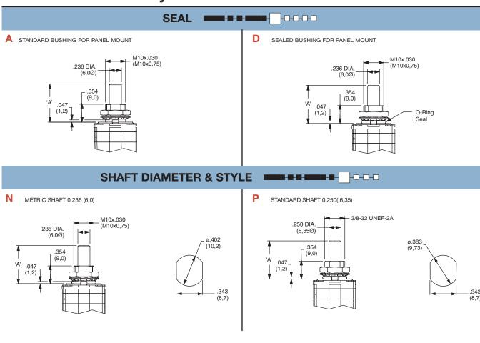
\*\*\*Note: Metric diameter shafts are only available with metric diameter bushings, standard 1.250 inch diameter shafts are only available with standard 3/8 diameter bushings.
