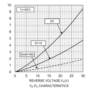
REVERSE POWER DISSIPATION:P<sub>R</sub>(W)
