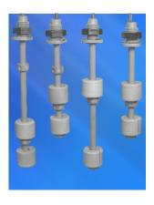
The two float range provide Make/Make, or Break/Break, switch action with a choice of 50 or 100mm separations. This type is particularly suitable for controlling filling or emptying of tanks via electromechanical relays.
