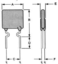
Lead Size: 24AWG, 0.51 mm Diameter
