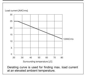
Note: the above indicated current ratings apply only for the RP.10 mounted with fins in the vertical orientation to allow airflow through the heatsink fins. For other mounting orientations please consult your Carlo Gavazzi Sales representative.
