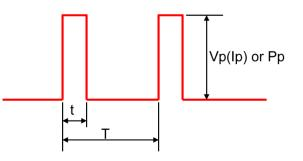
Where: Vp: Pulse limiting voltage (V)
