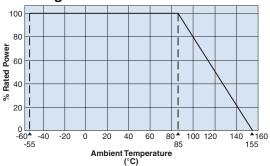
For resistors operated at an ambient temperature of 85°C or above, a power rating shall be derated in accordance with the above derating curve.
