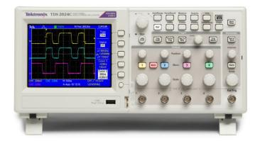
The TDS2000C Digital Storage Oscilloscope Series provides you with affordable performance in a compact design. Packed with standard features - including USB connectivity, 16 automated measurements, limit testing, data logging, and context-sensitive help - the TDS2000C Series oscilloscopes help you get more done in less time.
