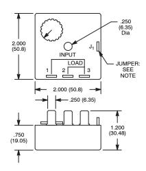
NOTE: 19–40 V AC or DC Cut J<sub>1</sub> for 40–288 V AC, DC
