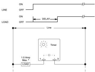
For higher current applications connect a switching relay in series with timer in place of load
