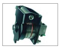
This Self Closing cap automatically protects the RJFTV square flange receptacle (MIL-DTL-3899 type), protecting your system from dust and water projection. A spring automatically closes the upper part of the cap when the RJFTV plug is removed from the receptacle.
