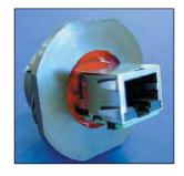
In some applications, a **transversal sealing** for the receptacle is a « must ». This will prevent fluids and dust from going through the receptacle when plug or cap are not mated to the receptacle. The sealed solution (version "S") has a compound at the rear of the receptacle as shown on the picture. For more information, please consult datasheet RJF-RJFTV Environmentally Sealed Receptacles, page 23.
