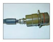
RJFTV series receptacles and plugs with EMI backshells provide a solution with 360° shielding: same protection than the one proposed per standard MIL-DTL-38999 serie III connectors. With those solutions we recommend using our reinforced and double shielded cat5E cable, see page 24.
