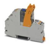
Pre-assembled relay module with push-in connection, consisting of: relay base, relay retaining bracket, and power contact relay with test button, integrated status LED, and freewheeling diode. Contact type: 1 PDT. Input voltage: 24 V DC
