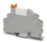
Pre-assembled relay module with push-in connection, consisting of: relay base with ejector and multi-layer gold contact relay. Contact type: 1 N/O contact. Input voltage: 24 V DC
