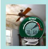
Extech's RH35 monitors Humidity, Temperature, and Dew Point for the previous 24 hours and alerts users to indoor mold hazard conditions starting with a frown icon warning when humidity reaches 60%RH. When the RH exceeds 65%, a loud audible alarm and bright flashing red LED will be triggered. The frown icon will also appear if the environment is too dry (<40%RH) where static electricity becomes a concern.
