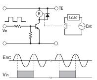
voltage and dropout voltage, depend on the ripple factor. Connect a smoothing capacitor for better operating characteristics as shown below.
