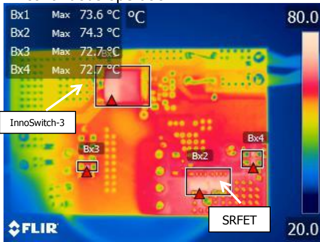
Figure 108 – 130 VDC 2.5 A Full Load. Temperature of InnoSwitch3-AQ: 73.6 °C. Temperature of SR FET: 74.3 °C. Ambient Temperature: 28.5 °C.
