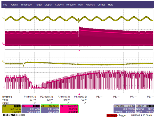
Figure 139 – DM Surge. V_{DS(MAX)} = 702 \text{ V} .
