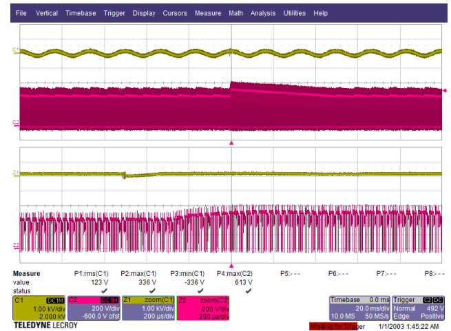
Figure 140 – CM Surge. V_{DS(MAX)} = 613 \text{ V}
