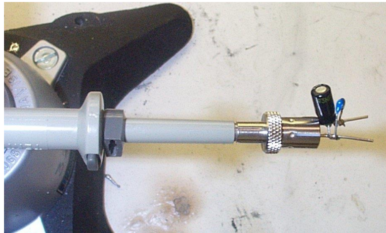
Figure 104 – Oscilloscope Probe with Probe Master ( www.probemaster.com ) 4987A BNC Adapter. (Modified with wires for ripple measurement, and two parallel decoupling capacitors added.)
