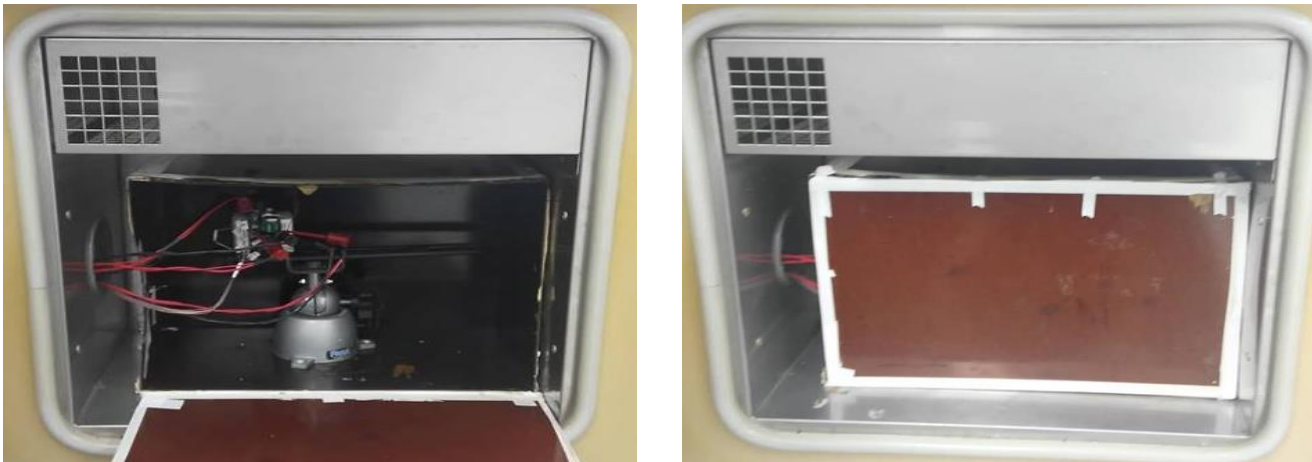
Figure 74 – Thermal Performance Set-up Using Thermal Chamber.
