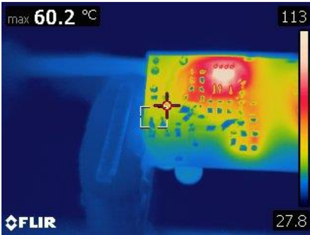
Figure 43 – BR1 – Bridge Rectifier Diode. Spot: 60.2 °C.
