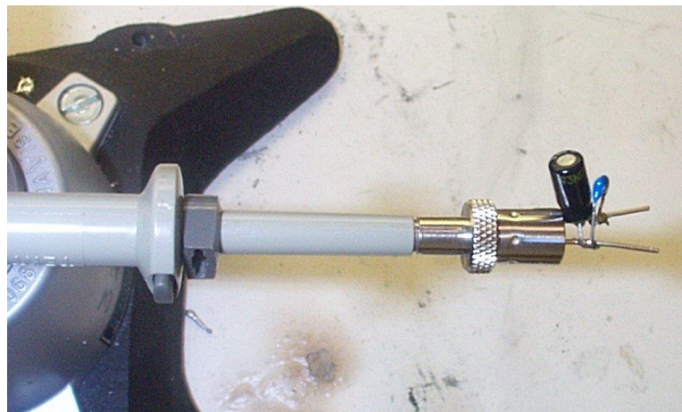
Figure 33 – Oscilloscope Probe with Probe Master 5125BA BNC Adapter. (Modified with wires for probe ground for ripple measurement, and two parallel decoupling capacitors added)
