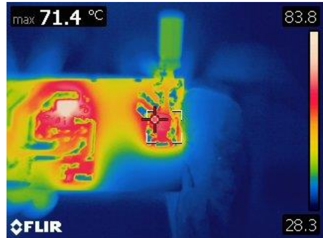
Figure 40 – D3 – Output Diode. Spot: 71.4 °C.
