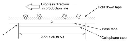
No lifting for the direction of progressing
