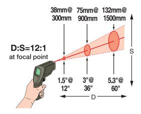
Use the ST20 XB within six feet of the intended target. At greater distances, the measured area will be larger (approximately the distance divided by twelve).
