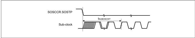
Figure 2.6 Sub-clock oscillation start timing
