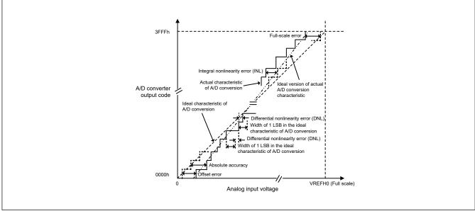
Figure 2.42 Illustration of A/D converter characteristic terms
