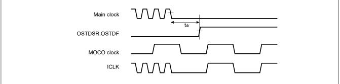
Figure 2.43 Oscillation stop detection timing
