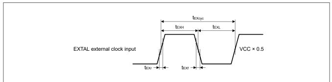
Figure 2.3 EXTAL external clock input timing
