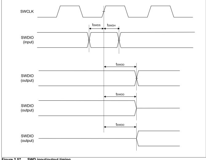
Figure 2.57 SWD input/output timing
