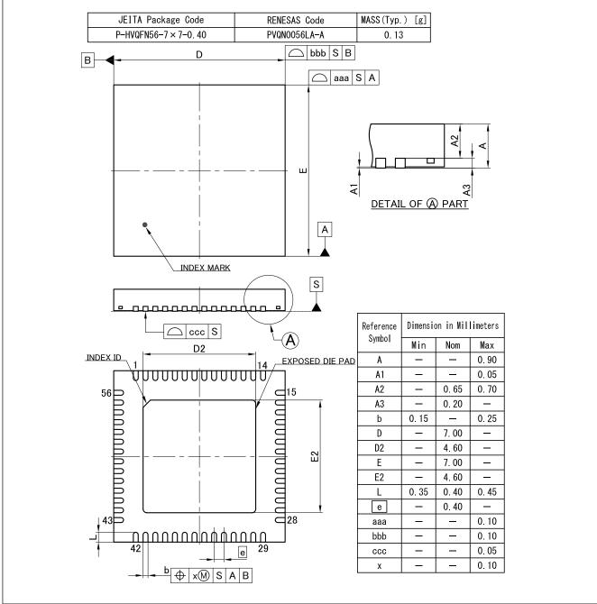
Figure 2.5 QFN 56-pin
