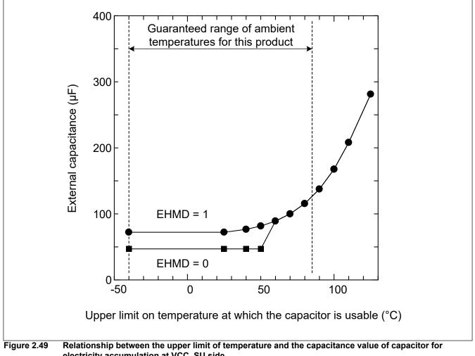
electricity accumulation at VCC\_SU side
