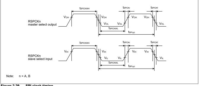
Figure 2.29 SPI clock timing
