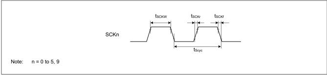
Figure 2.21 SCK clock input timing
