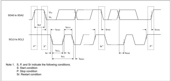
Figure 2.38 I2C bus interface input/output timing
