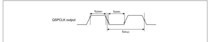
Figure 2.36 **QSPI clock timing**
