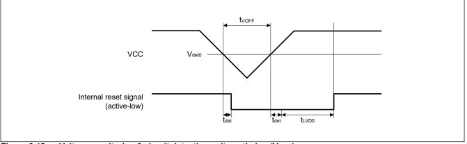
Figure 2.45 Voltage monitoring 0 circuit detection voltage timing (V<sub>det0</sub>)
