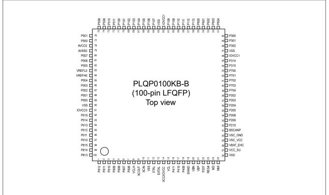
Figure 1.2 Pin assignment for LFQFP 100-pin
