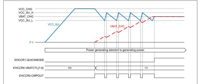
VBAT\_EHC pin charging operation during high-speed startup function period of EHC capacitor Figure 2.48 charging
