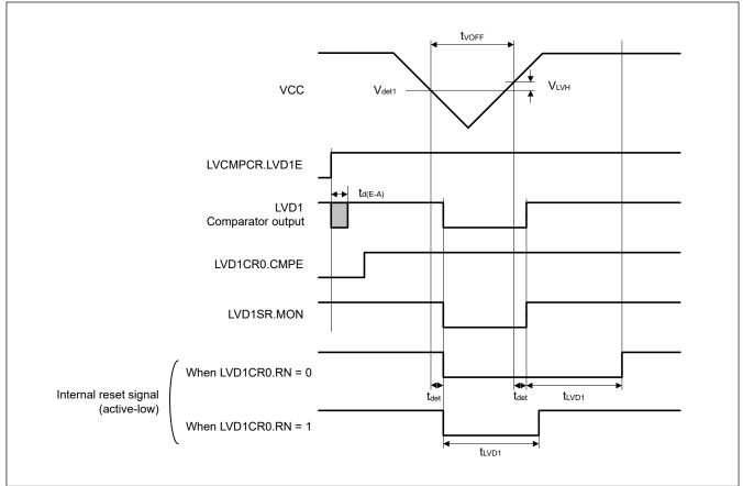
Figure 2.46 Voltage monitoring 1 circuit detection voltage timing (V<sub>det1</sub>)
