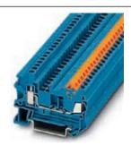
Feed-through terminal block, Connection type: Quick connection, Screw connection, Cross section: 0.25 mm<sup>2</sup> - 1.5 mm<sup>2</sup>, AWG :24- 16, Width: 5.2 mm, Color: blue, Mounting: NS 35/7,5, NS 35/15
