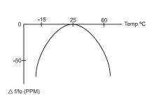
To calculate the frequency stability the parabolic curvature constant (K) is needed. For calculating the stability at 45°C?
