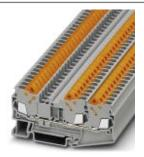
Feed-through terminal block, Connection method: Quick connection, Cross section: 0.5 mm<sup>2</sup> - 2.5 mm<sup>2</sup>, AWG: 20 - 14, Width: 6.2 mm, Height: 37.8 mm, Color: gray, Mounting type: NS 35/7,5, NS 35/7,5
