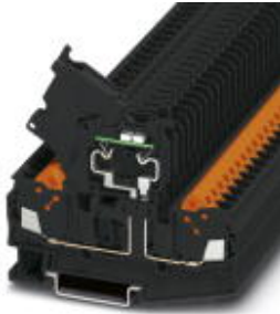
Fuse terminal block for assembly on NS 35, for 5 x 20 cartridge fuse inserts
