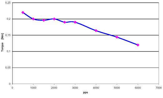
Figure 5.1: QSH4218-35-10-027 speed vs. torque characteristics
