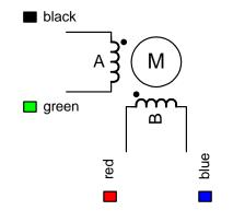
Figure 4.1: Lead wire configuration
