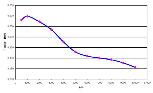
Figure 5.2: QSH4218-41-10-035 speed vs. torque characteristics
