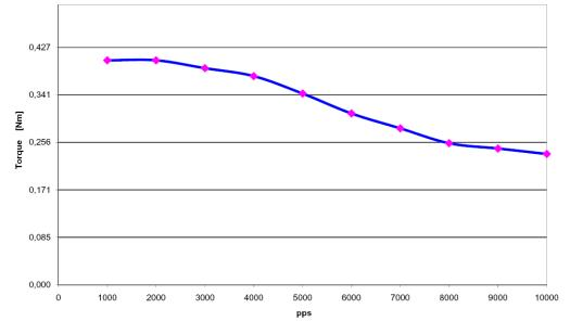
Figure 5.4: QSH4218-47-28-040 speed vs. torque characteristics
