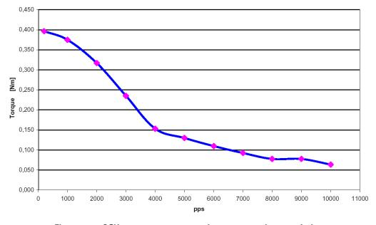
Figure 5.3: QSH4218-51-10-049 speed vs. torque characteristics
