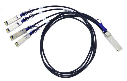
Volex's QSFP28 passive breakout Direct Attach Cables feature 4 transmitting and 4 receiving channels at 25Gbps per channel speed and support 100Gbps (QSFP28) to 2x 50Gbps (2x QSFP28) and 4x 25Gbps (4x SFP28) breakout configurations. The cable assemblies meet 25GbE Ethernet (IEEE 802.3by) standard with substantial signal integrity margin providing high performance and bandwidth interconnect solutions for high-density applications.
