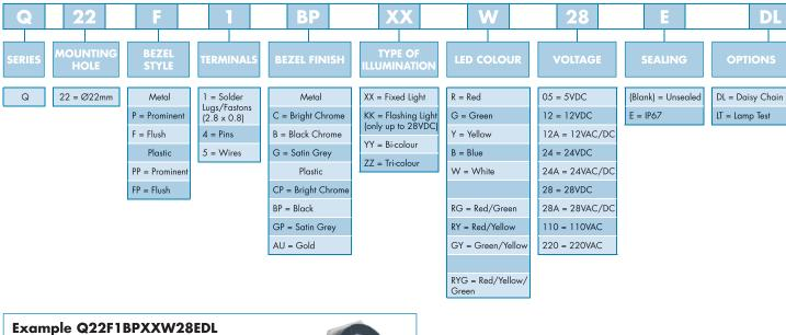
Ø22mm, flush bezel, solder lug terminals, black plastic finish, fixed light, white, 28volt DC LED, IP67 Panel Seal, Daisy Chain
