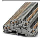
Double-level terminal block, connection method: Push-in connection, cross section: 0.14 mm<sup>2</sup> - 4 mm<sup>2</sup>, AWG: 26 - 12, width: 5.2 mm, color: gray, mounting type: NS 35/7,5, NS 35/15
