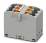
Distribution block, Basic terminal block, nom. voltage: 500 V, nominal current: 24 A, connection method: Pushin connection, number of connections: 6, cross section:0.14 mm² - 4 mm², AWG: 26 - 12, width: 15.6 mm, height: 21.2 mm, color: gray, mounting type: adhesive
