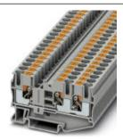
Feed-through terminal block, Connection method: Push-in connection, Cross section: 0.5 mm<sup>2</sup> - 10 mm<sup>2</sup>, AWG: 20 - 8, Width: 8.2 mm, Height: 42.2 mm, Color: gray, Mounting type: NS 35/7,5, NS 35/15
