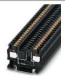
Fuse modular terminal block, Connection method: Push-in connection, Cross section: 0.2 mm<sup>2</sup>- 6 mm<sup>2</sup>, AWG: 24 - 10, Nominal current: 10 A, Nominal voltage: 24 V, Width: 6.2 mm, Fuse type: Type F (miniature), Fuse type: Flat, Mounting type: NS 35/7,5, NS 35/15, Color: black
