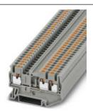
Feed-through terminal block, Connection method: Push-in connection, Cross section: 0.14 mm<sup>2</sup> - 4 mm<sup>2</sup>, AWG: 26 - 12, Width: 5.2 mm, Height: 35.2 mm, Color: gray, Mounting type: NS 35/7,5, NS 35/15
