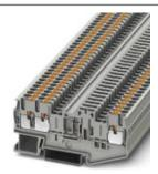
Disconnect terminal block, Connection type: Push-in connection, Cross section: 0.14 mm² - 4 mm², AWG: 26 - 12, Nominal current: 16 A, Nominal voltage: 400 V, Length: 81.9 mm, Width: 5.2 mm, Color: gray, Assembly: NS 35/7,5, NS 35/15
